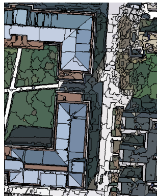
Figure 40: Outlines of objects created with 'multiresolution segmentation' algorithm.
